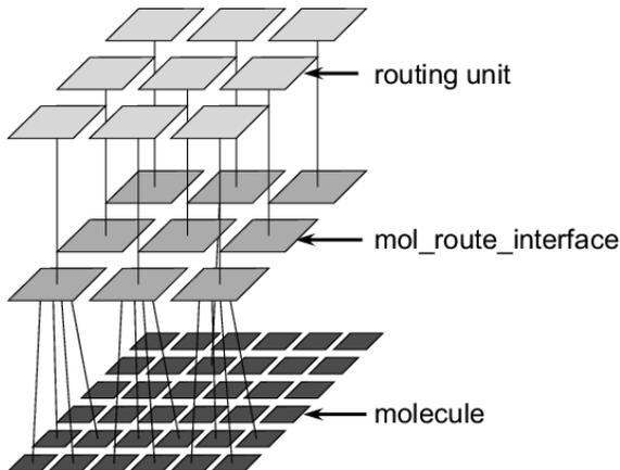
Figure 4. The tissue is actually composed of 3 layers: the molecules, the interface, and the routing units (not all connections are shown between molecules and interfaces).
